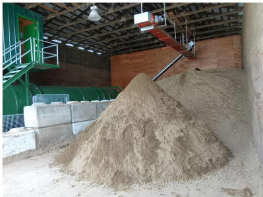
Figure 4 Compost bedding from drum composter
